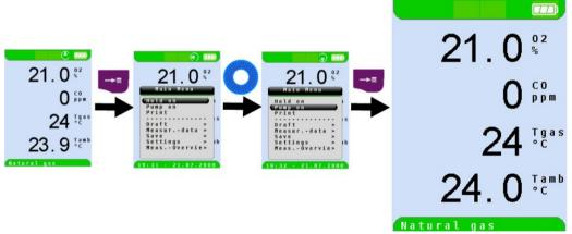
When the gas pump is switched off, the pump symbol is no longer shown in the status bar. Changes in the corresponding measured gas values cannot be ruled out, e.g. the O2 value may change as a result of lack of oxygen in the gas lines inside the device. If the gas pump remains off for a longer period of time, calibration in fresh air should be carried out before a new measurement is made.
