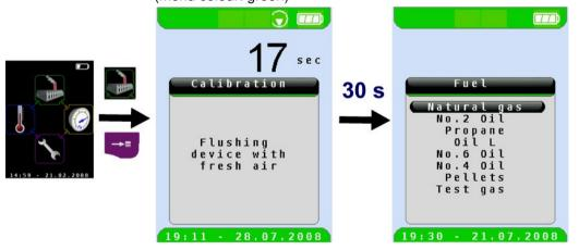
After a cold start the calibration phase takes 30 seconds. After calibration the last fuel used is selected by default and displayed for confirmation.
