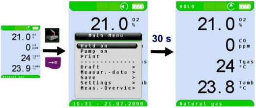
As soon as the flashing HOLD symbol is displayed in the status bar, all measured values (except draft) are held temporarily.
