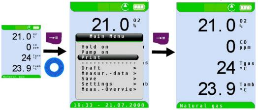
Measured values which were not in HOLD mode prior to the print command are current values or "momentary values". These values are printed immediately upon activation of the print command.
